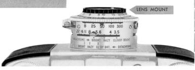
You'll get sharper pictures if you carefully estimate the distance in feet from the lens to the main subject; then set the lens at this distance. To bring the camera into focus, turn the LENS MOUNT until the camera-to-subject distance is opposite the focus-index mark.
